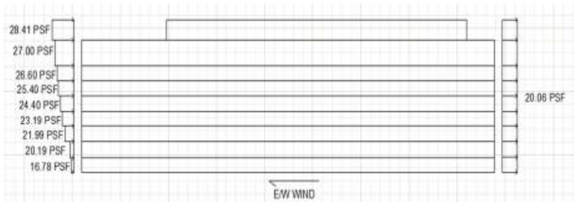
FIGURE 9: THIS FIGURE GRAPHICALLY SHOWS THE WIND PRESSURES ON THE BUILDING IN THE EAST/WEST DIRECTION.
