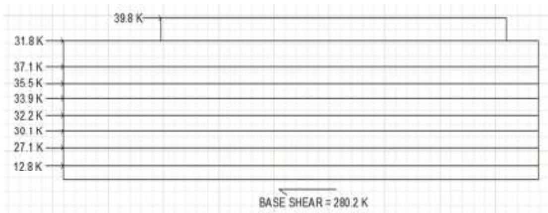
FIGURE 10: THIS FIGURE GRAPHICALLY SHOWS THE WIND SHEAR FORCE ON EACH STORY IN THE EAST/WEST DIRECTION.
